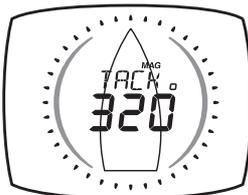
The compass heading that the vessel will follow should it tack through the wind, calculated by the display. Apparent wind angle and magnetic heading must be available for this calculation to be made.
