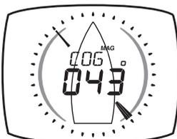
The vessel's course over the ground as calculated by the GPS Antenna.
