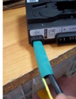
Figure 11: Detail of double insulated connection
